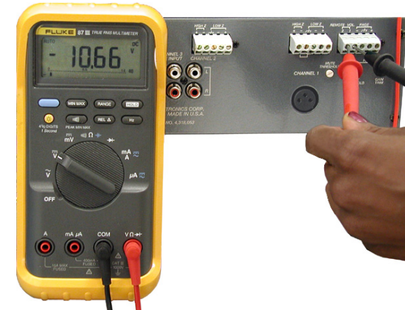
Measuring control voltage for a Peavey UMA™ 35T II: meter leads are oriented incorrectly relative to the amp's terminals
